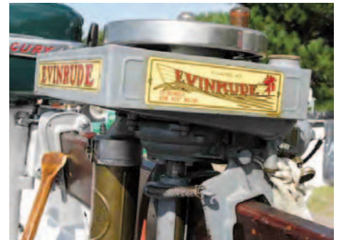
The upper unit of an early teens Evinrude rowboat motor.
